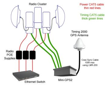
high at the site location. The Mini-GPS2 simply needs to be able to view satellites to receive synchronization. In addition, consider the exposure to lightning when placing it near other radio equipment. The GPS antenna needs to be connected before applying power.
